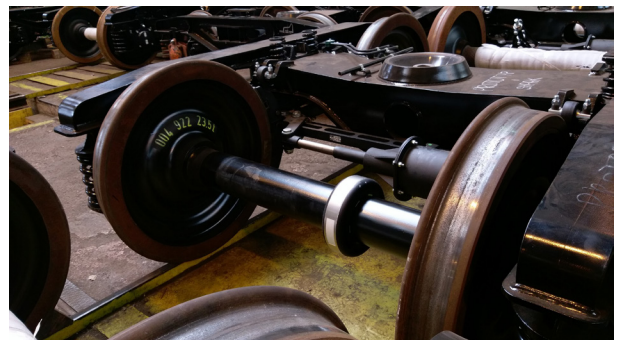
Photo from AxleRing installation
